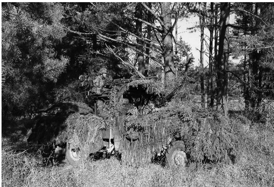
Figure 1. Netherlands reconnaissance truck camouflaged with natural materials in a concealed position.
